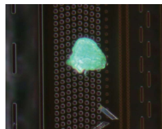
MIX: Fluorescence + Darkfield Both the IC pattern and residue are clearly represented.
